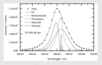
Fig. 1: Measured and fitted Titanium neutral emission line with individual components of the fit function
