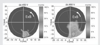
Fig. 1: Chromium concentration map for the low power case (a) and the high power case (b)
