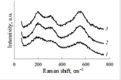
Fig. 1. Raman spectra of films TiN, deposited at current density 32 mA/cm2 and flow of N2 (sccm): 1 – 2; 2 – 4; 3 – 6;
