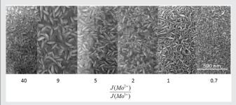
SEM micrograph of the film morphology as a function of the ion flux ratio of Mo2+ and Mo1+.
