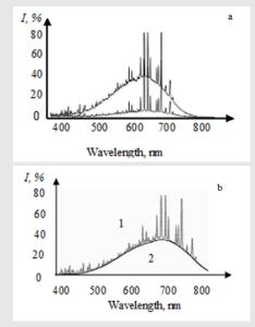
Fig.1. a – Typical emission spectra at different discharge power; b – Extraction of the thermal radiation spectrum (1 - initial spectrum, 2 – extracted spectra of thermal radiation).
