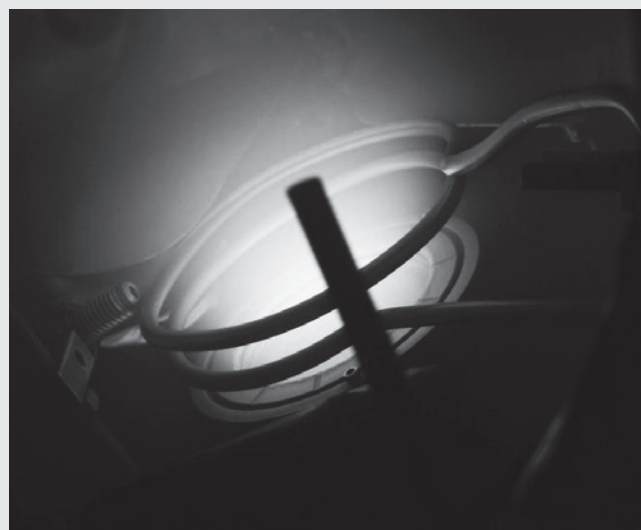
Figure 1: Image of an ICIS plasma with a 76.2 mm diameter copper target and 80 mm copper RF-coil.
